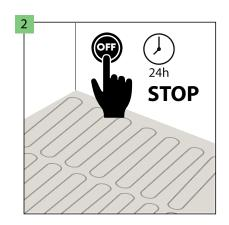
Before their installation the panels must be subjected to the 24-hour acclimatisation at the temperature of 18–30°C, in the premises where they will be installed. In the event of transport or/and storage at the temperature below +5°C, the time acclimatisation must be extended to 48 hours
