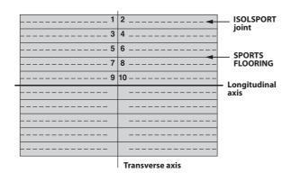
Once the flooring is in position, Isolsport will stuck-down (in strips of 20 cm) around the peripherie and the entire breadth of all doorways and accesses of the sports hall with a Polyurethane adhesive.
